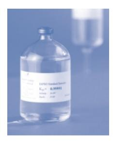
IAPSO Standard Seawater is available in sealed glass bottles, each containing ca.200ml of natural seawater. The bottle label carries information on its conductivity ratio (K15) and salinity according to the Practical Salinity Scale 1978 (PSS78).
